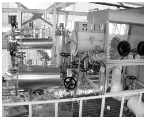
The LBE loop is mainly composed of a main test loop, bypass loop for filtering LBE and a mixture-gas supplying system. The liquid metal in the main test loop circulates in the following order: electromagnetic pump (EMP) – EM flow meter – oxygen controller – test section – magnetic filter – EM pump. Major specifications of the KAERI's loop are summarised in Table 1.
