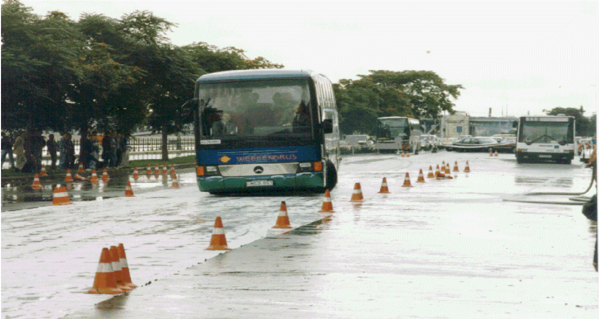
Figure 15. Lane change and braking on a slippery road
