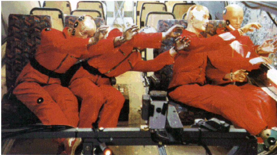
Figure 12. Illustration showing the efficiency of a two-point safety belt during a test-run of the overturning sideways of a coach
