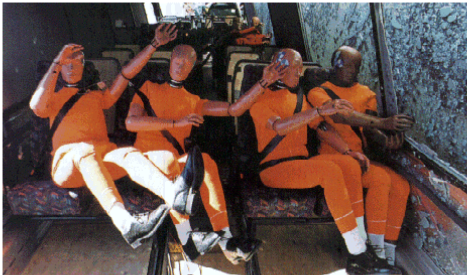
Figure 13. Illustration showing the efficiency of a three-point safety belt during a test-run of the overturning sideways of a coach
