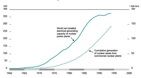
Figure 5. Installed power of nuclear power plants and their cumulative generation of radioactive waste
