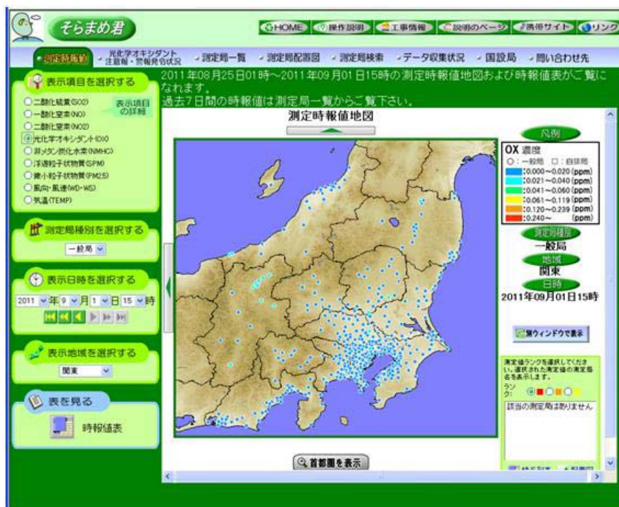
Figure F.2: Presentation of a GIS-based system for air pollutants and an example of monitoring stations and results (oxidant level in stations in Kanto region): Part 2
