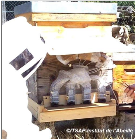
Capture at the hive entrance Hive is equipped with the RFID system (MAJA 13.56 MHz, Microsensys, GmbH, Germany)
