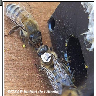
Tagged bee on flight board RFID reader with tunnel to scan labelled bees entering/exiting the hive (MAJA 13.56 MHz, Microsensys, GmbH, Germany)
