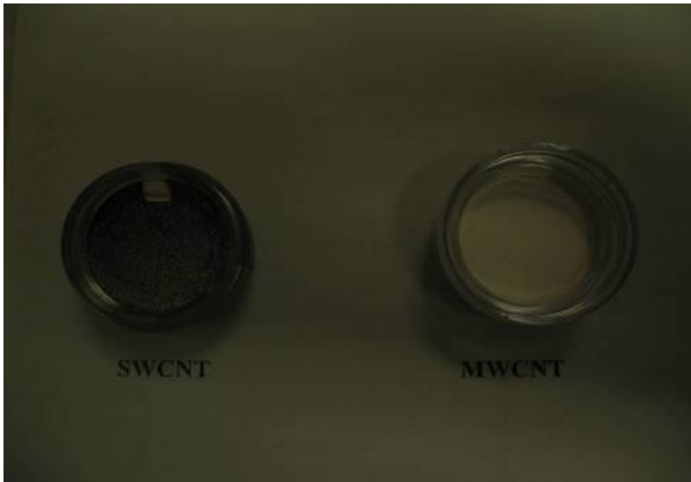
Figure 40. Photograph of the open face cassettes containing the filters used to capture nanotubes. The SWCNT filter on the left shows significantly more particle deposition than the MWCNT filter on the right.
