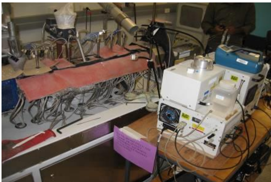
Figure 12. Configuration of measurement equipment, with sampling manifold, relative to the location of the extruder machine.
