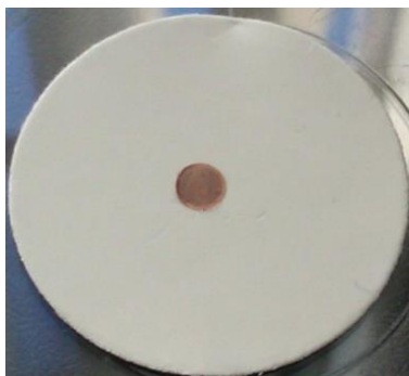
Figure 4: Carbon coated TEM copper grid on a MCE filter
