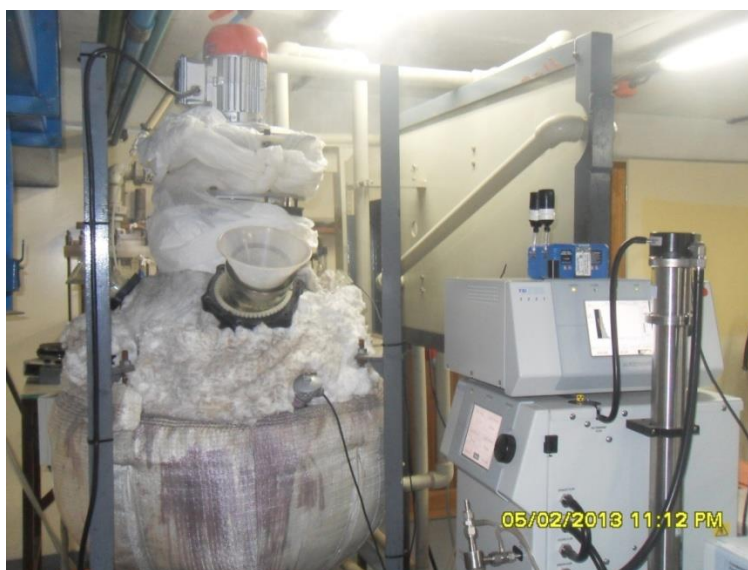
Figure 2: Chemical reactor with real –time measurement instruments, SMPS and APS, with occupational hygiene pumps on top
