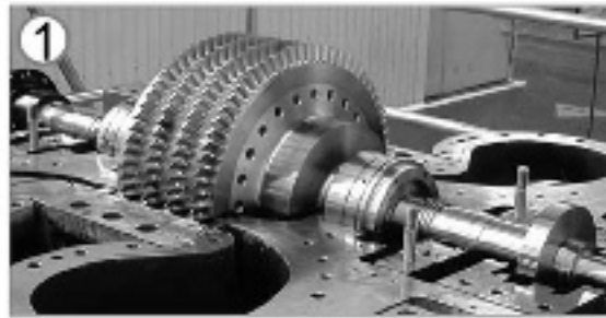
Figure 13. Test compressor of 1/3 full scale
