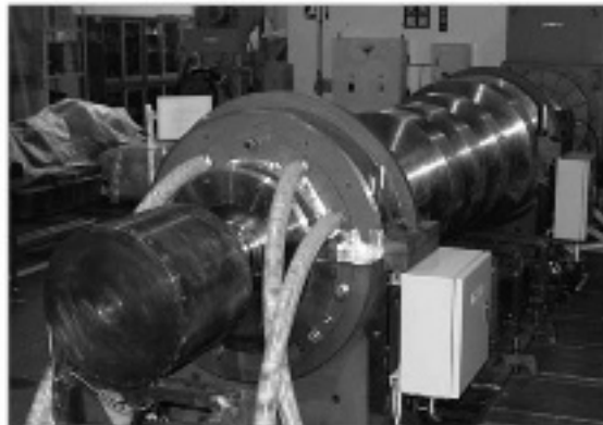
Figure 14. MB rotor test rig of 1/3 full scale
