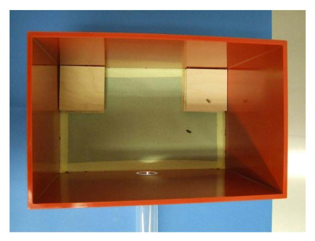
Figure 2 Arenas for testing cockroach baits: harbourage unit of dual chamber box, top view
