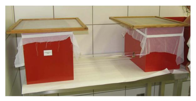
Figure 1. Arenas for testing cockroach baits: dual chamber box with rectangular units, side view
