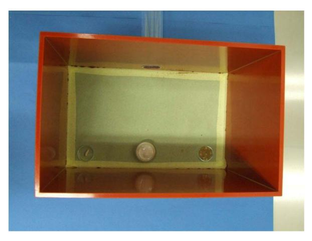
Figure 3 Arenas for testing cockroach baits: feeding unit of dual chamber box, top view.
