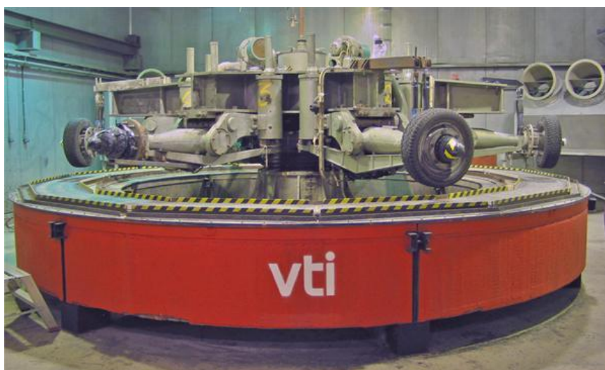
Figure 0.7 Road simulator in VTI
