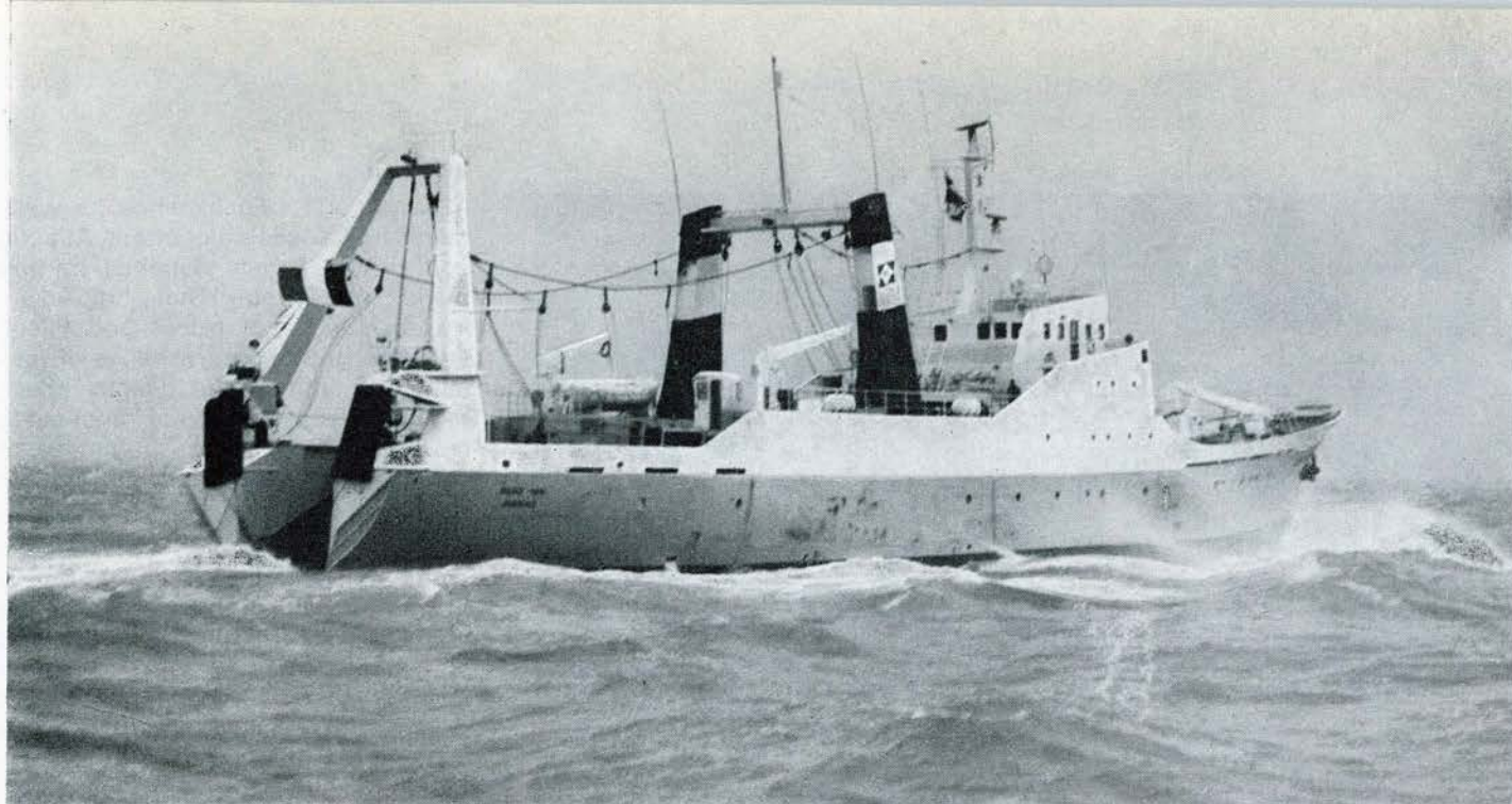
A modern French stern-trawler, the Pierre Vidal, which has facilities for freezing and salting.
