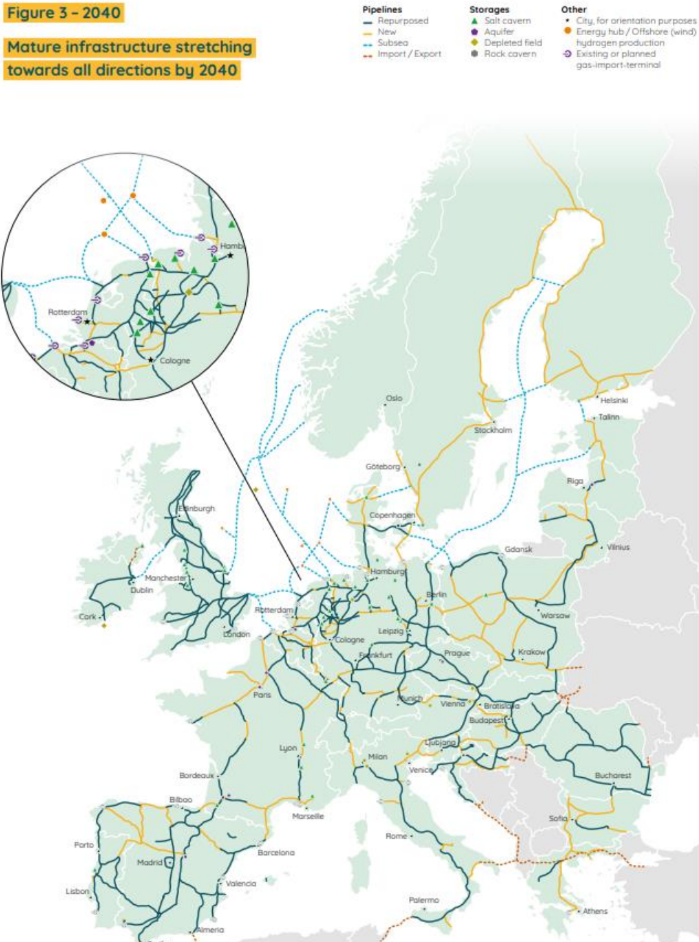
Figure 3.14. Repurposed pipelines can connect Hamburg to a European hydrogen network by 2040
