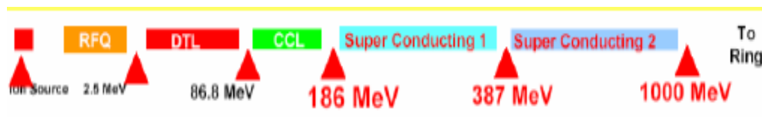
Figure 1. Schematic layout of the SNS linac
