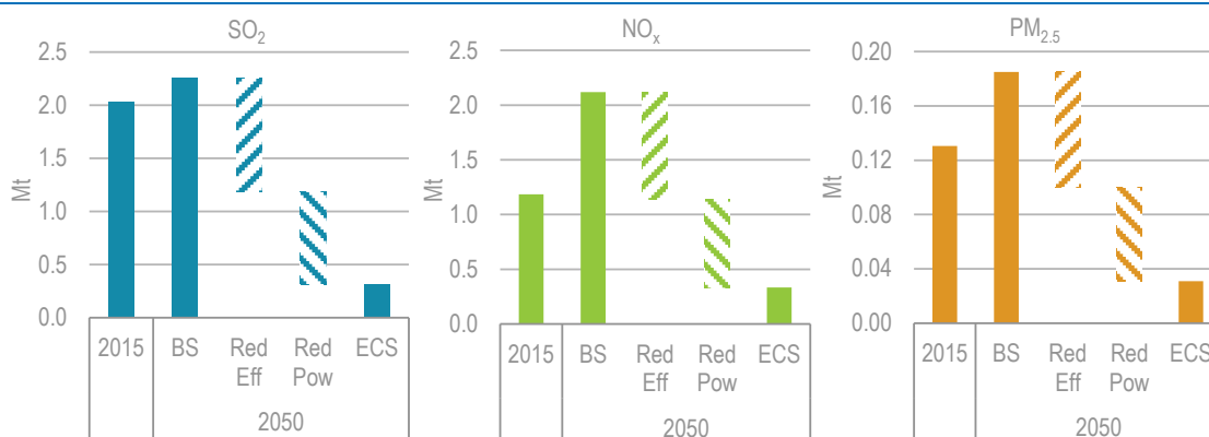
Figure 3.22 • Reductions in air pollutant emissions linked to space cooling by type of pollutant
