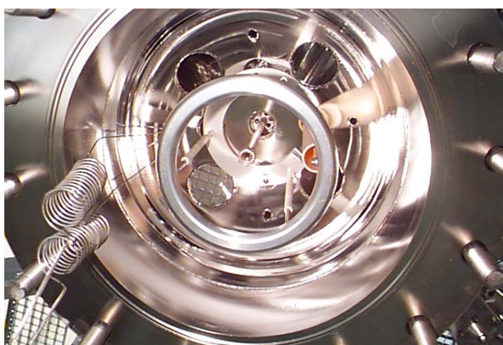
Figure 4. The inside of the upper lid of the PCV showing from left to centre: internal thermocouples, glow discharge electrode, inspection window and inlet tube for gas treatment
