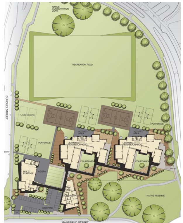
Figure 3. Site plan. The school is structured in two main complexes or learning neighbourhoods linked by all-weather walkways.
