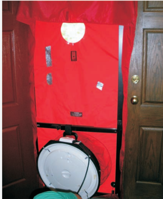
Figure 3.14 Blower door test apparatus
